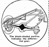
only when travelling on a curve, and you will see that immediately there is a difference of speed between the two it is accommodated by the planet wheels, C, revolving on their bearings.
